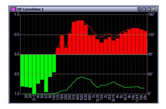
It gives you a very good impression what happens to the phase depending on the frequency. It's well-suited to check reverb units, stereo extender and any kind of compression like mp3 or even to just check what's going wrong with your mix or master.
