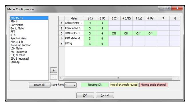
Here, instruments are added and removed and the physical audio inputs of the selected audio device are routed to the inputs of the individual instruments.
